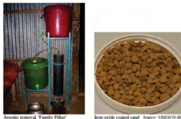
Figure 20: Iron Oxide Coated Sand Filter
