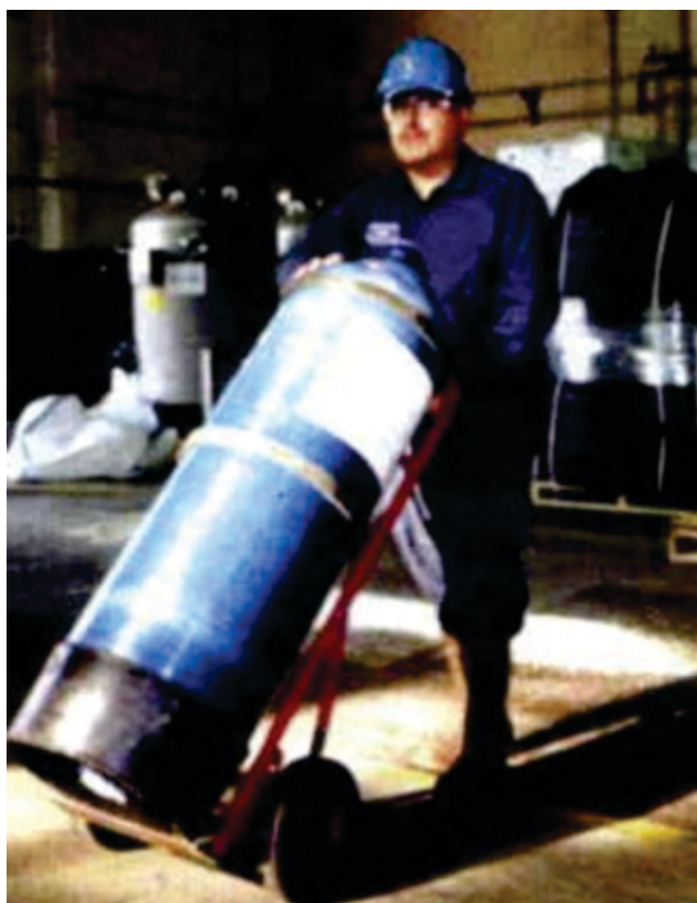
Figure 94: Siemens Ion Exchange Resin Canister
