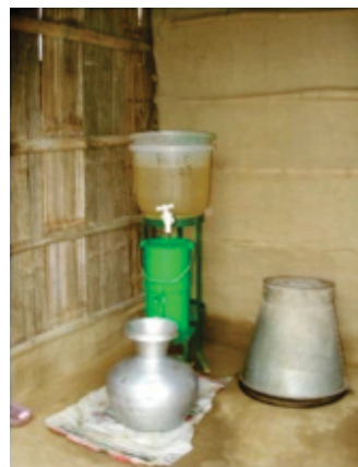
Figure 14: Read-F Arsenic Removal Unit
