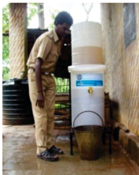
Figure 57: Household Iron Removal - CSIR - NEERI Technology
