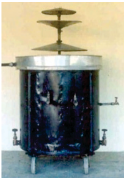
Figure 61: Water Iron Removal Unit of DRDO
